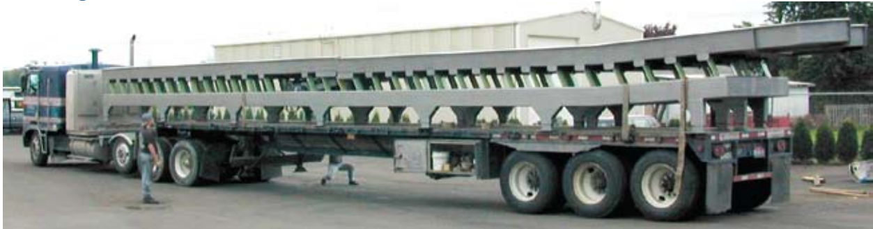
This vibrating conveyor design was originally developed for sawmill duty. Manufactured for a seed processor, this conveyor is 3' wide and over 60' long. Conveying speed is approximately 80' per minute. Capacity of 125 tons per hour is routine.
