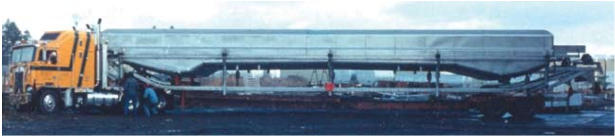
This is GEM's first high volume deluge blancher. At sixty-nine feet overall length, it was considered enormous when it was manufactured in 1982. Today, transporting a new GEM French fry potato blancher requires more than one large truck.
